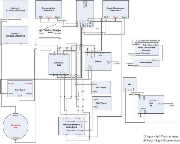
Figure 1. Electronics System Diagram
